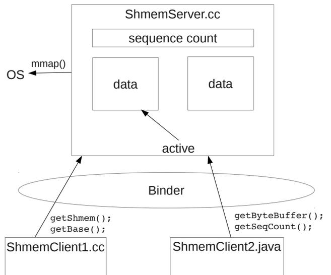
FIG. 3. The shared-memory server `ShmemServer` allocates a shared region. Native as well as Java processes can get a reference to the region via Binder remote method invocation and afterwards access it directly for data exchange.
