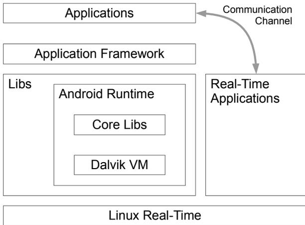
FIG. 1. Architecture diagram of our real-time Android implementation.
